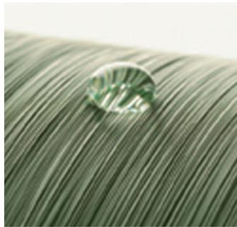
Fort Wayne Metals provides PTFE<sup>1</sup> based coatings and coating compositions on wires for a variety of medical applications. LubriSkin™ and DuraSkin™<sup>2</sup> PTFE dispersion coatings are applied to medical wires to
