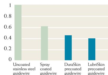
The graph above shows relative physical resistance of coated wire passing through human tissue according to coating type.
