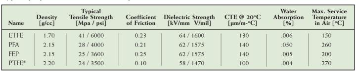
These properties are for reference only and can vary significantly dependent on processing conditions and material grade \*PTFE is not a melt-processable thermoplastic.
